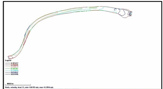
Fig. 12: Velocity distribution as contour lines in x-y Plane at level 11"Water Surface"
